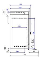
Electrical inlet (power) ΕI Refrigerant Outlet RO
